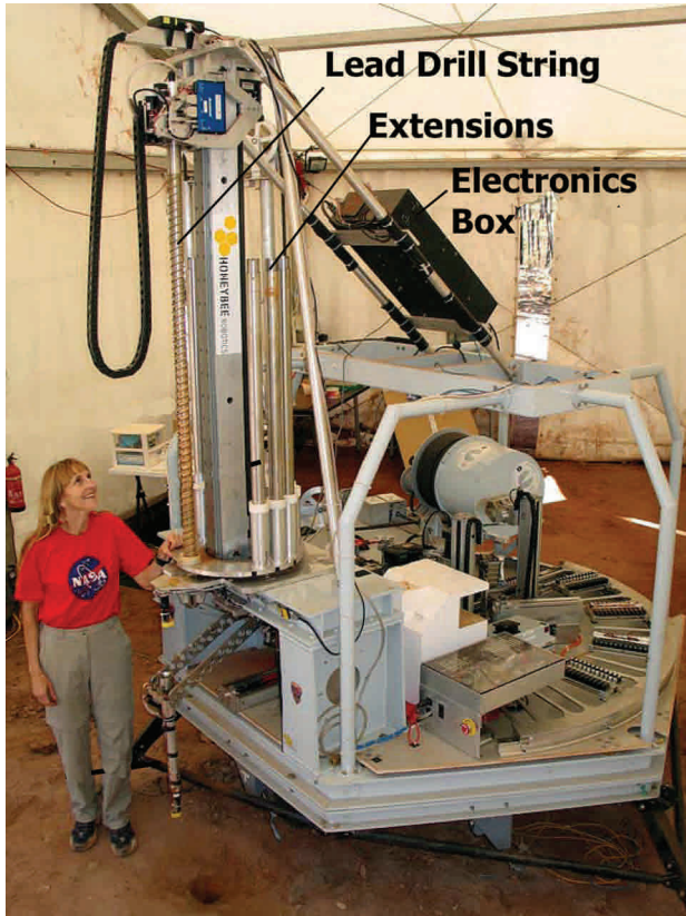
FIG. 5. A photograph of the MARTE drill mounted on the lander.
