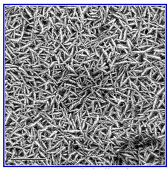
**Figure 3.** SEM micrograph of a film with composition  $Bi_{0.10}Sb_{0.90}$ . The features are characteristic of all the films deposited at -1.02 V vs Ag/AgCl (3 M NaCl) for 1 h.
