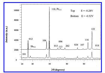
**Figure 4.** XRD patterns of 200-nm Bi/Sb wire arrays deposited at E = -0.52 V and -0.28 V vs Ag/AgCl from a bath of 0.06 M Bi and 0.02 M Sb. The Miller indices indicate the alloy peaks. The peak widths are narrower for the slower growth conditions (E = -0.28 V), indicating a more homogeneous sample.
