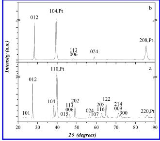
**Figure 2.** XRD patterns of two  $\text{Bi}_{1-x}\text{Sb}_x$  films. The films were obtained from two solutions: (a) 0.02 M Bi<sup>3+</sup> plus 0.06 M Sb<sup>3+</sup>; and (b) 0.06 M Bi<sup>3+</sup> plus 0.02 M Sb<sup>3+</sup>. The depositions were carried out at E = -1.02 V vs Ag/AgCl (3 M NaCl) for 1 h. The film compositions are Bi<sub>0.95</sub>Sb<sub>0.05</sub> and Bi<sub>0.10</sub>Sb<sub>0.90</sub>, respectively, as determined by EPMA.
