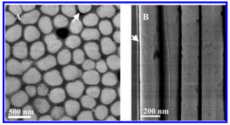
**Figure 6.** SEM nanowires of  $Bi_{0.85}Sb_{0.15}$  nanowires: (a) bottom view after removal of the Pt electrode by mechanical polishing; and (b) cross-section or edge view. The lighter regions are the wires. They are dense. The filling of each pore is very high, yet does not completely fill the pores in all regions (gap marked with an arrow). Nucleation and growth of wires occurs in greater than 95% of the pores.
