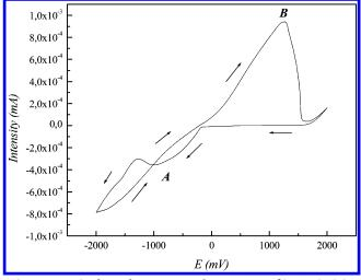
Figure 1. Cyclic voltammetry of 0.040 M  $Bi^{3+}$  – $Bi(NO_3)_3$ ·  $5H_2O$ – plus 0.040 M  $Sb^{3+}$  – $SbCl_3$ –. Scan rate, 0.01 V/s<sup>-1</sup>; reference electrode, Ag/AgCl (3 M NaCl); temperature, 25 °C.
