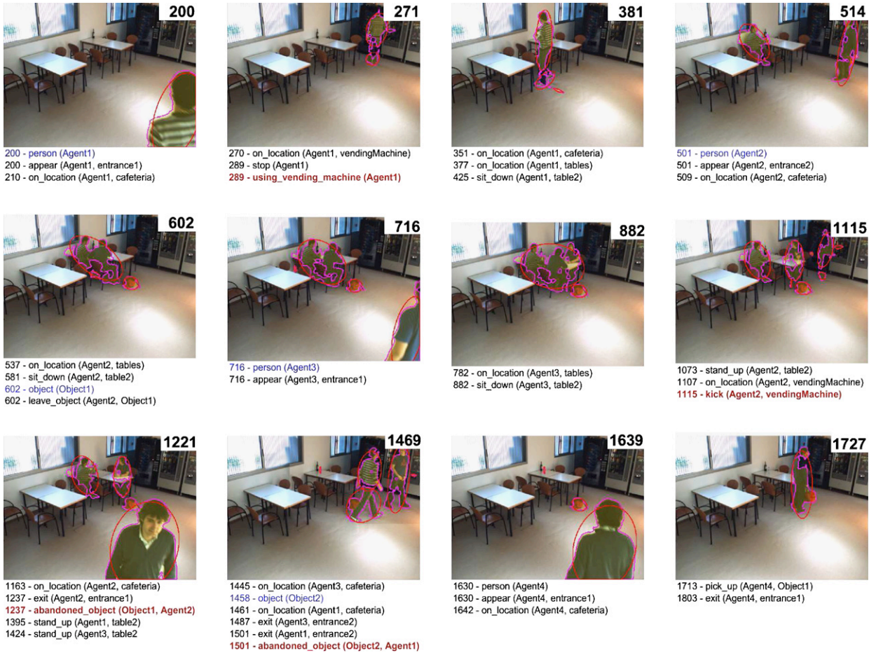
Fig. 11. Set of semantic annotations produced for the indoor scene, which have been automatically generated for the fragment of recording comprised between frames 150 and 1839.
