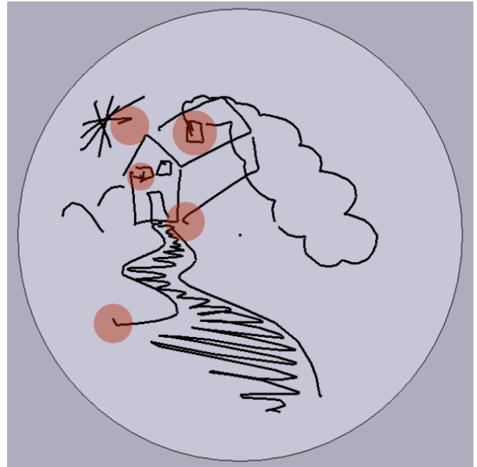
Fig. 6. A drawing generated using the presented prototype as a touch pad. Dry friction in the ball-and-socket joints induce some artifacts at the end of the strokes (indicated with shadowed circles).
