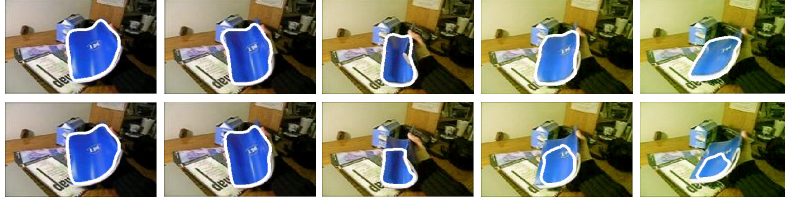
Fig. 4. Tracking results of a bending book in a sequence with smooth lighting changes. Upper row: using the proposed method the tracking works. Lower row: using only a contour particle filter and assuming smooth change of color the method fails.
