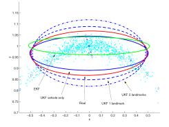
Figure 1: In red (x): actual mean and covariance; in green (+): linear transformation of mean and covariance; in blue (\*): nonlinear transformation of mean and covariance for robot only; in blue dashed  $(\Box)$ : nonlinear transformation for robot and one landmark; in blue dash dot  $(\diamond)$ : nonlinear transformation for robot and 2 landmarks.
