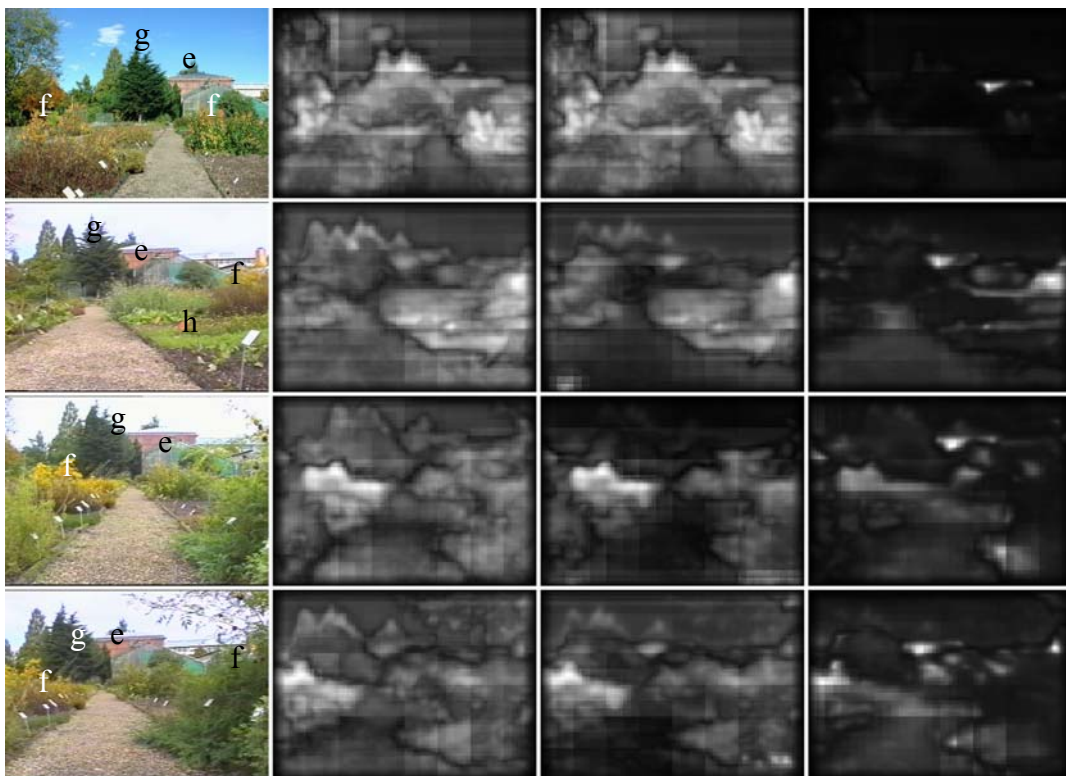
Figure 2: Visual saliency computed for scene “B” for four different illumination conditions. Note that there are slight changes in perspective between the images. Each source image (left column) was processed with lighting intensity normalization (second column), lighting intensity and illuminant color normalization (third column), and color ratios (fourth column). The whiter regions indicate the more salient parts detected. In the source images the following things are indicated: (e) red house, (f) yellowish bushes, (g) trees, and (h) red sign. The other signs, similar in shape as the red one, are white.
