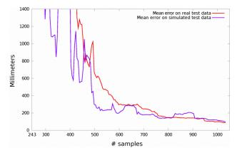
Fig. 5. Exact learning on real data recorded with 5DOF and a training set of 1000 samples and test set with 500 samples. The measured errors (violet) are compared to simulated values with noise  $\sigma_{err} = 20 mm$  (red).
