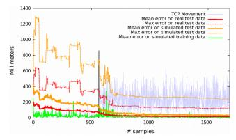
Fig. 7. Comparison of the incremental learning progress when processing real data from marker tracking (orange) and simulation w/o noise (red). Thick lines represent mean errors and dotted lines maximal errors. After 600 training experiences no new data is acquired but previously learnt data is processed anew in arbitrary order. The difference between the TCP positions is shown (light blue).
