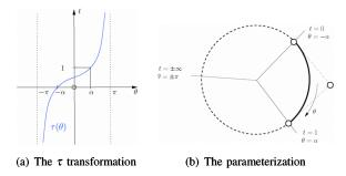
Fig. 2. Transformation from a joint angle to the corresponding parameter of the Bézier form.
