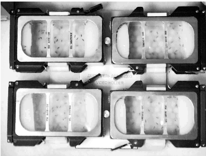
Fig. 1. Miniaquaria with flies (lower frame). Image from the flight video recording. Above a larger view of the container. Dimensions of the type I container: 9.0 x 4.0 x 2.5 cm.
