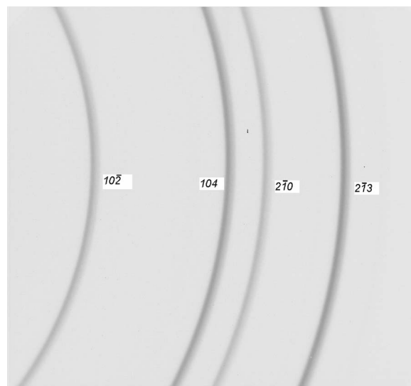
FIG. 2. WAXS pattern of alumina obtained in the low resolution arrangement ( D=20 cm), at 2\theta_{\min}=22.0^\circ and with an accumulation time of 30 s.
