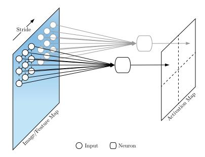
FIGURE 2.4: An example of how a single filter is implemented in a convolutional neural network.
