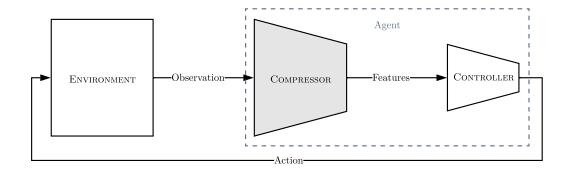
FIGURE 5.1: A recap of the role of the compressor in agents that use a compressorcontroller design.
