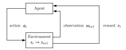
FIGURE 2.10: The basic agent interaction loop in reinforcement learning. Modified from Francois-Lavet et al. (2018).
