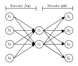
FIGURE 2.5: A simple undercomplete autoencoder. In the process of learning to reconstruction its inputs  $\boldsymbol{x}$ , it encodes the most important features of the data for achieving this in the encoding  $\boldsymbol{z}$ .
