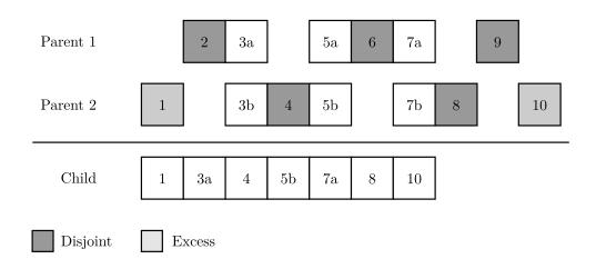
FIGURE 2.9: A visualisation of the crossover operation between two parent genomes. Each box represents a connection gene, labelled by innovation number. Parent 2 is fitter, and therefore the excess and disjoint connection genes are inherited from them. Genes with matching innovation numbers are inherited randomly from either parent.
