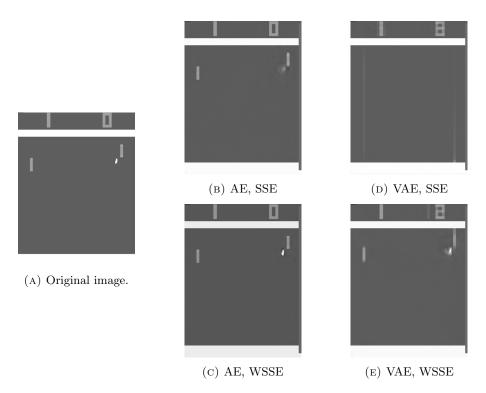
FIGURE 5.14: A comparison between the image reconstruction quality for different Pong models that use the DQN-inspired architecture and a representation size of 30. (A) Shows the original image, (B) and (C) the AE candidates using SSE and WSSE respectively, and (D) and (E) the VAE candidates using SSE and WSSE respectively.
