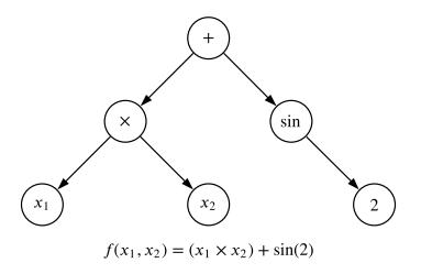
FIGURE 2.7: An example of a function represented by an abstract syntax tree.
