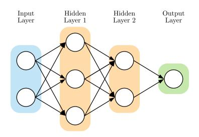
FIGURE 2.1: An example of a multilayered feed-forward neural network with two inputs, a single output, and two hidden layers.
