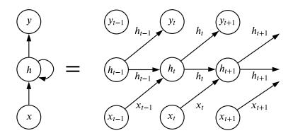
FIGURE 2.3: An example of the how the values of the inputs, hidden state, and outputs in a recurrent neural network are propagated over time.
