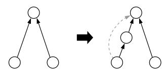
FIGURE 2.8: A visualisation of the add node mutation operator for NEAT
