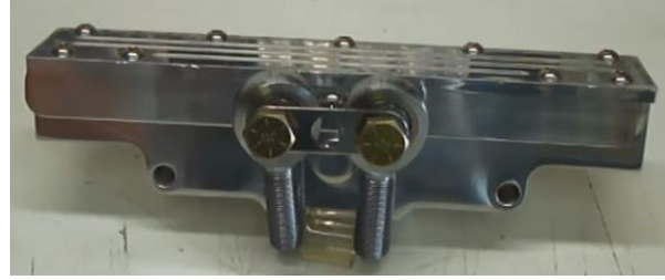
Figure 2.97: Selected rack and pinion, rear view
