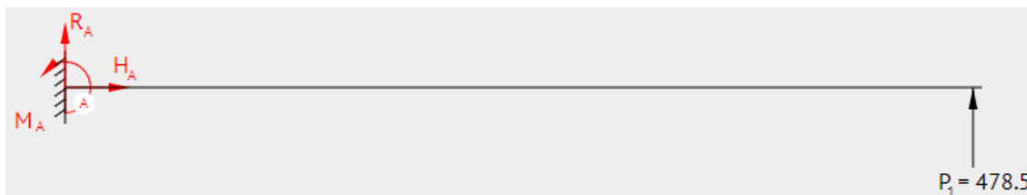
Figure 2.81: Free body diagram of the rear trailing arm under maximum lateral loading
