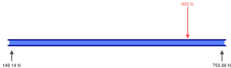
Figure 2.80: Bending forces acting on the trailing arm
