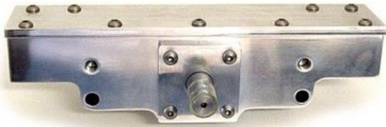
Figure 2.96: Selected rack and pinion, front view
