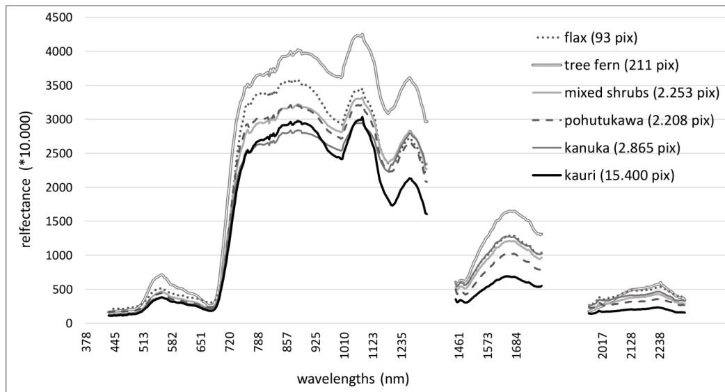
Figure II-7 Mean spectra of kauri (black) and five other canopy species (grey) that have the highest separabilities from the kauri spectrum in this study (see Table II-A2). The number of pixels (pix) used to generate the mean spectra is given in parentheses.
