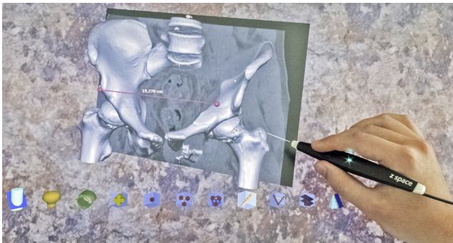
Fig. 4 3D interface showing the zSpace display with stylus interaction. A model extracted from the CT dataset is shown along with the anatomical plane, and the 3D buttons at the bottom of the screen.
