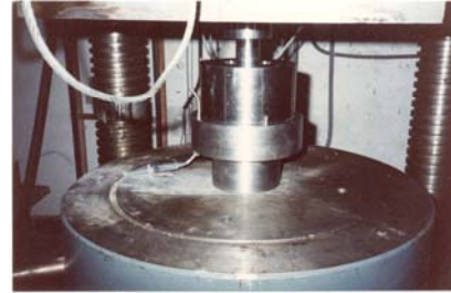
Figure 4. Extracted Pore Solution Equipment
