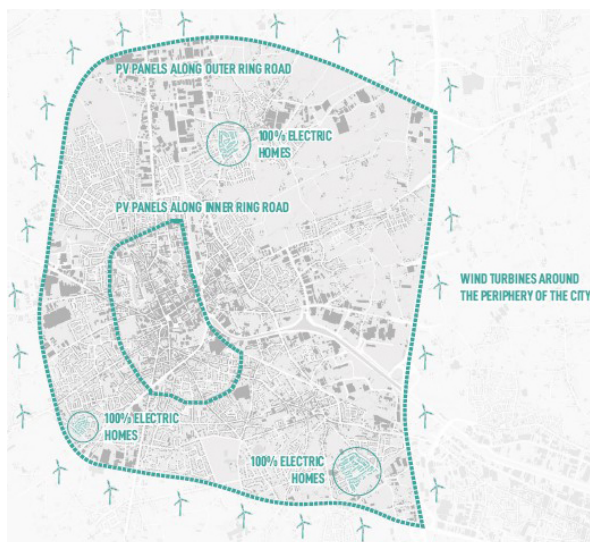
Figure 8: The energy production plan for the city including two rings of photovoltaic panels alongside highways, a ring of wind turbines, three 100% electric communities in addition to rooftop and ground-based photovoltaic panels.
