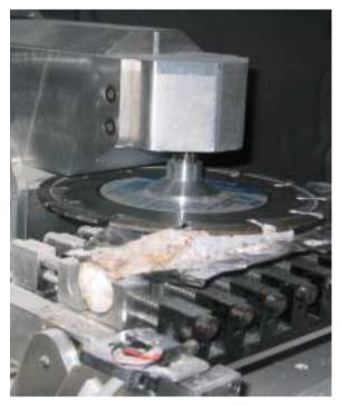
Figure 8: CSHS Facing Saw. The Facing Saw creates a clean flat surface on the top of the core for improved sensing
