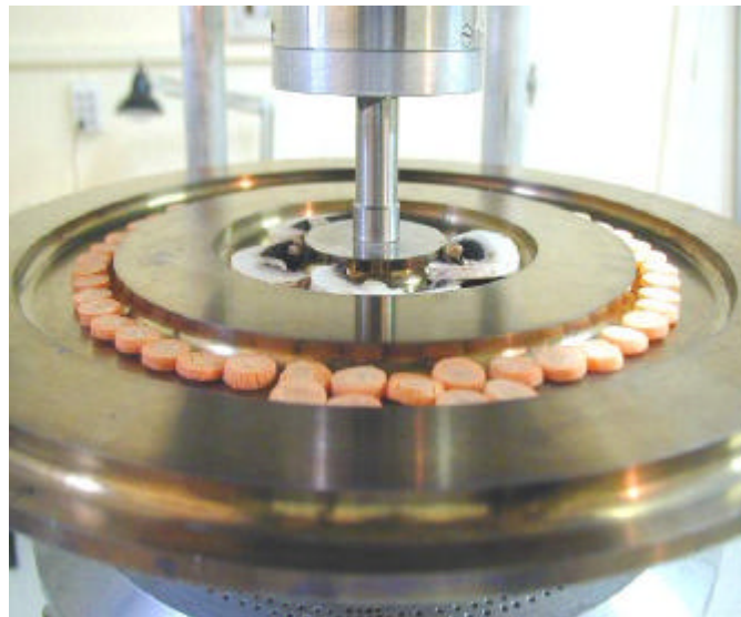
Figure 2. Carrot and mushroom dehydration by applying simple direct contact ultrasonic vibration and forced-air.
