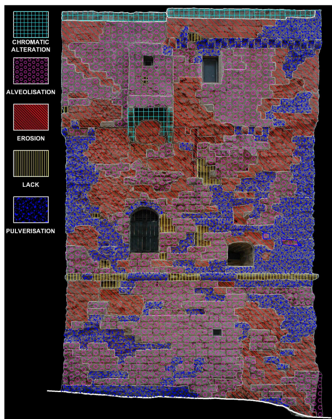
Figure 7. Representative decay map of Marina Serra Tower.
