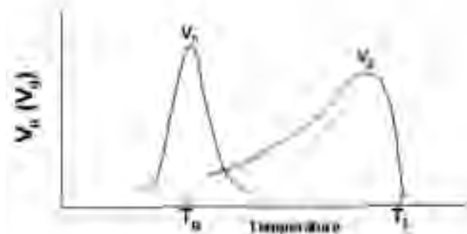
Fig. 4- Sketch of the rate of crystal nucleation ( V_n ) and growth ( V_g ) as a function of temperature. T_L denotes the liquidus temperature and T_g the glass transition temperature.
