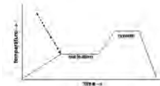
Fig. 5- Simplified scheme of the two-step thermal treatment used to obtain a glass-ceramic material.
