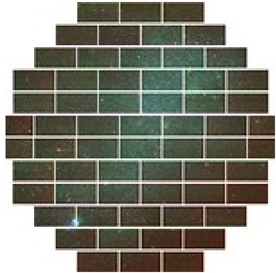
Fig. 2: Blanco telescope - DECam camera has 64 mosaic CCDs available to make the capture.
