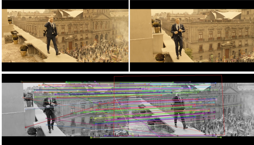
Fig. 1.11: Local feature extraction and matching for computing the homography between a pair of frames (i.e. how the image on the left should be translated to match the one on the right), that subsequently allows motion detection and estimation. Note: frames were extracted from the opening scene of the “Spectre” movie.
