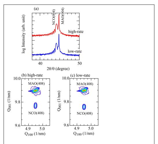
Figure 1: (a) X-ray  $2\theta/\theta$  diffraction profiles for the high-rate film and the low-rate film. (b and c) Reciprocal space mappings around the (408) MgAl<sub>2</sub>O<sub>4</sub> reflection for the high-rate film and the low-rate film.
