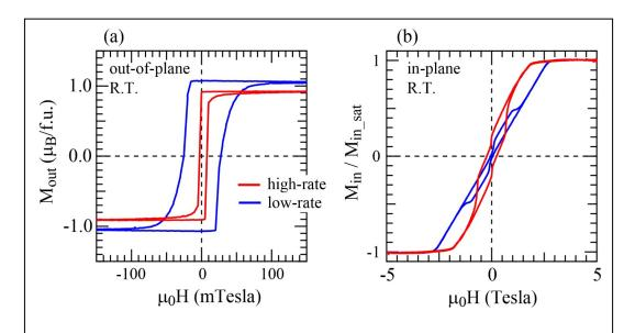
Figure 2: Room-temperature magnetic field dependence of the (a) out-of-plane and (b) in-plane magnetization for the high-rate film (red) and the low-rate film (blue). In (b), the magnetization is normalized by the magnetization value at 5 Tesla.
