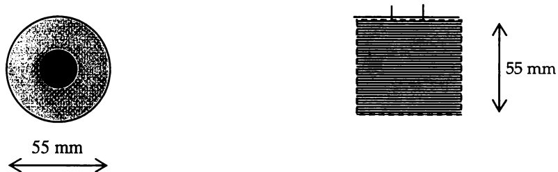
TMC tube nozzle with bolt in the centre, profile and side - view
