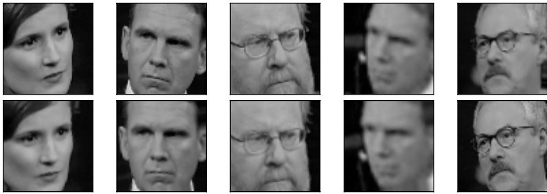
Figure 4, upper row: Examples of leant heads, leading to in-plane rotation of the face. The lower row shows the same faces after they have been rotated back to an upright position by Videana 's face recognition system using the detected position of the eye region. This step is important for a later comparison of two faces.
