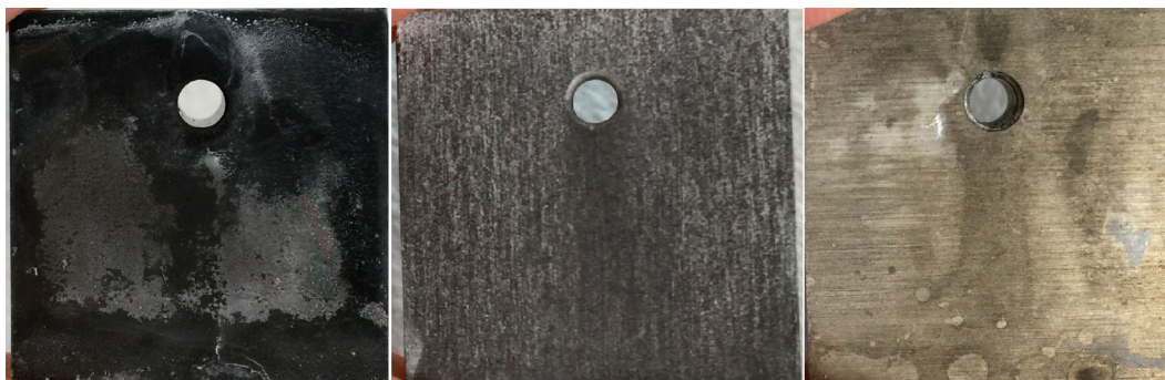
Figure 4. Corrosion Test Week 2, (L) Superhydrophobic, (M) Superhydrophilic, (R) Untreated.
