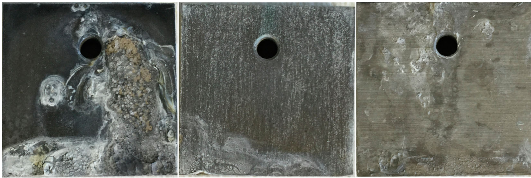
Figure 9. Corrosion Test Week 6, (L) Superhydrophobic, (M) Superhydrophilic, (R) Untreated.
