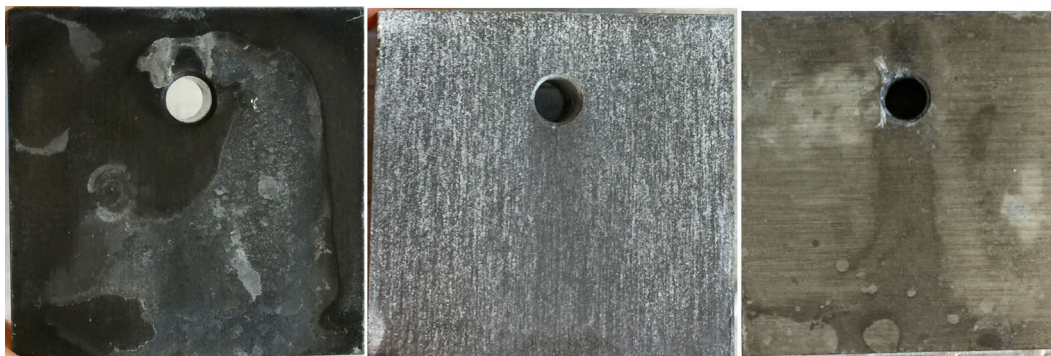
Figure 5. Corrosion Test Week 3, (L) Superhydrophobic, (M) Superhydrophilic, (R) Untreated.
