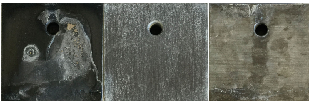
Figure 6. Corrosion Test Week 4, (L) Superhydrophobic, (M) Superhydrophilic, (R) Untreated.
