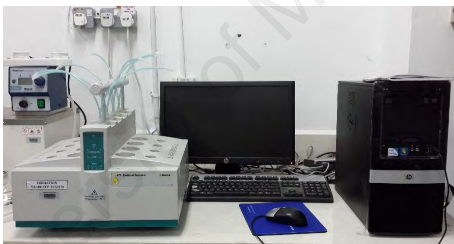
Figure 3.3: Metrohm-873 Biodiesel Rancimat
