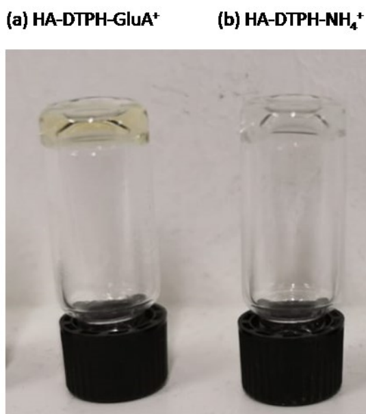
Figure 23 Inverted tube assay for HA-DTPH-GluA + (a) and HA-DTPH-NH 4 + (b). Both hydrogels, showed a solution (flow) – gel (no flow) transition under argon atmosphere at RT after 24 hours of incubation.
