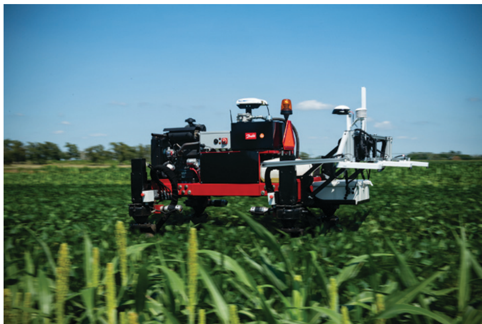
Figure 3. Flex-Ro, a 60 HP UGV, collecting soybean plot information. (Photo credit: Santosh Pitla, University of Nebraska-Lincoln.)
