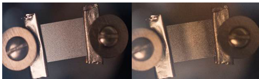
FIG. 1. A GaAs crystal mounted between two electrical terminals, with (left) no frosting, and (right) frosting produced by heating above 657 °C. The foil sandwiched between the terminal washers and the crystal are used to improve the uniformity of electrical contact for ohmic heating.
