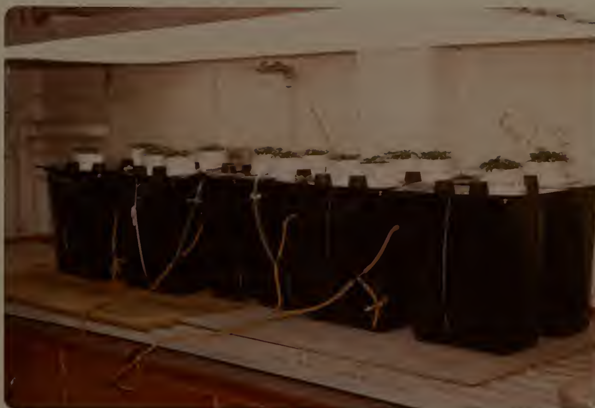
Figure 4.--Arrangement of 20-liter cans and cut-and-inverted 1-liter yogurt cups used for primary root growth studies on selected crop species in controlled subsurface nutrient solutions.
