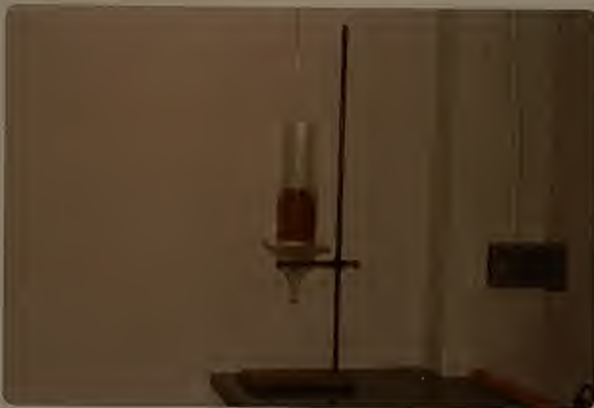
Figure 3.--Specially constructed Plexiglass column for displacing subsoil solutions for subsequent chemical analyses.
