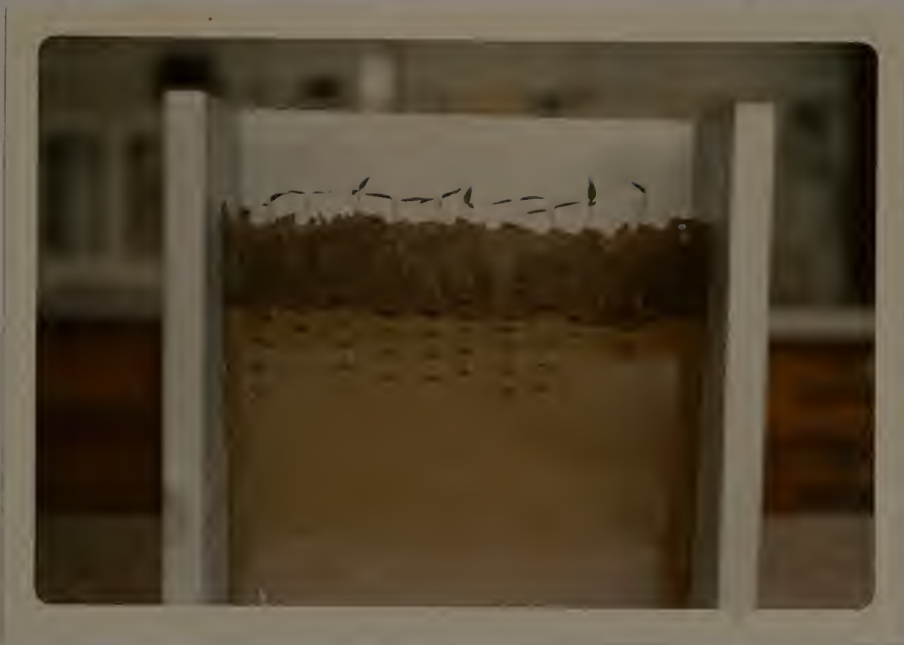
Figure 1.--Glass-front box used in vertical split-root technique for the periodic observation of primary roots in situ .
