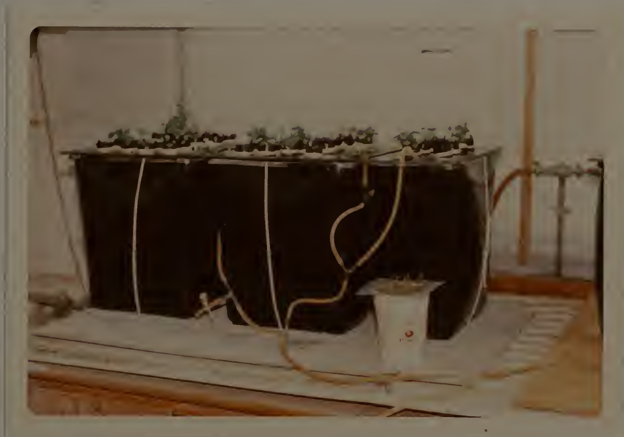
Figure 2.--Arrangement of 20-liter plastic cans used for preliminary primary root growth studies on six crop species in culture solutions.
