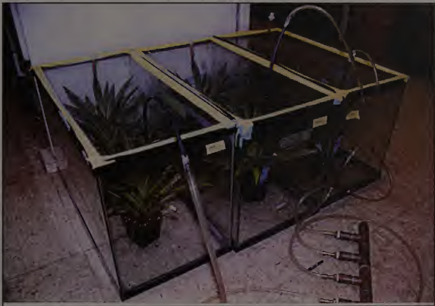
Figure 2 : Flow-through system for ethylene treatment. For each treatment plants were placed in three 36-l sealed tanks. Ethylene was provided at a flow rate of one air exchange per hour and at a concentration of 100 \mu\text{l}\cdot\text{l}^{-1} .
