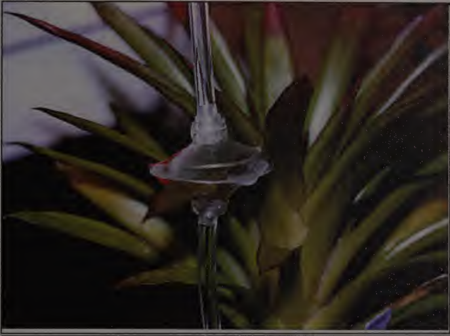
Figure 3 : Ethylene treatment on one leaf, flow-through system. Eight-ml silicon chamber with an inlet and outlet is shown. A section of the leaf ( \sim 4.5 \text{ cm}^2 ) was placed in the chamber and exposed to constant flow of 100 \mu\text{l}\cdot\text{l}^{-1} ethylene.
