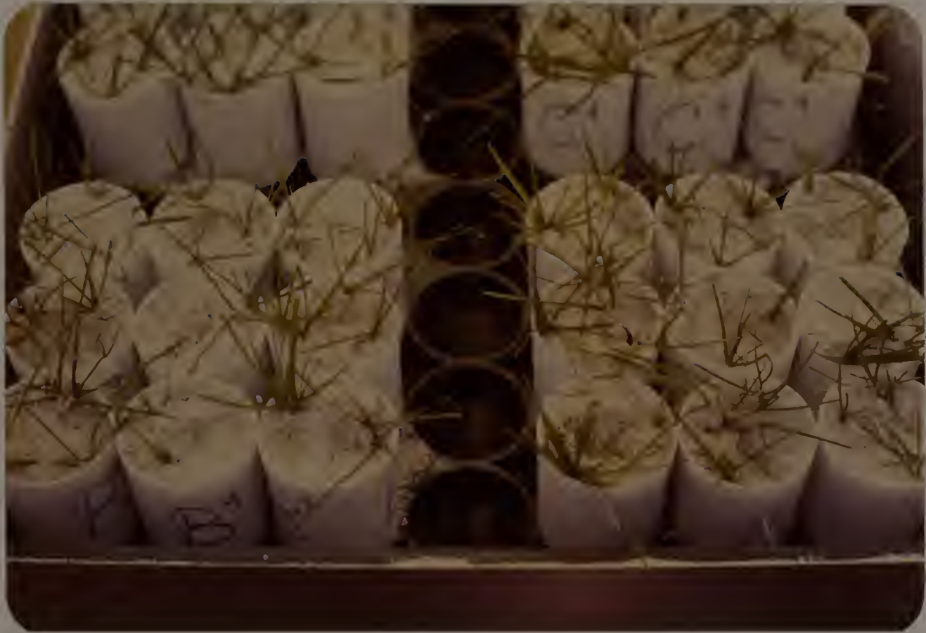
Figure 1. Arrangement of semi-conical tubes containing perennial ryegrass plants on support rack suspended over compartmentalized, plexiglas box.
