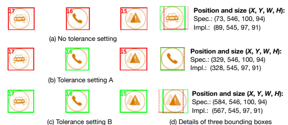
Figure 7. Flexible tolerance ( \Delta X, \Delta Y, \Delta W, \Delta H ) for examining bounding boxes. (a) No tolerance setting. (b) Tolerance setting A = (4, -1, 4, 4). (c) Tolerance setting b = (-1, -1, 4, 4). (d) Details of the bounding boxes.
