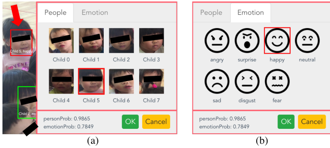
Fig. 6. An interactive method for users to correct an inaccurate label for the highlighted girl. The left-hand side (a) shows the interface for correcting face recognition results, while the right-hand side (b) shows the interface for correcting emotion recognition results.
