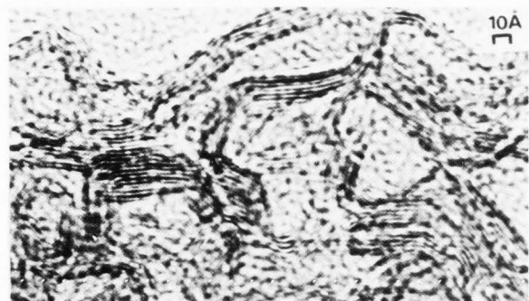
Figure 18 - 002 lattice fringe image showing porous microtexture in saccharose-coke heat-treated at 2800°C.
