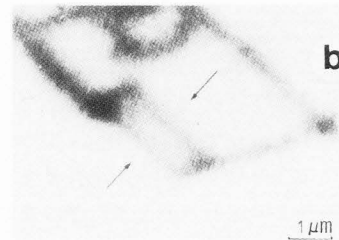
Figure 15. (a) Weak-beam TEM and (b) SEM EBIC micrographs of dislocations in deformed Si. The arrows indicate the widely separated partial dislocations of a dissociated screw dislocation. There is no EBIC contrast due to the stacking fault between them. (After Ourmazd et al (1983a)).
