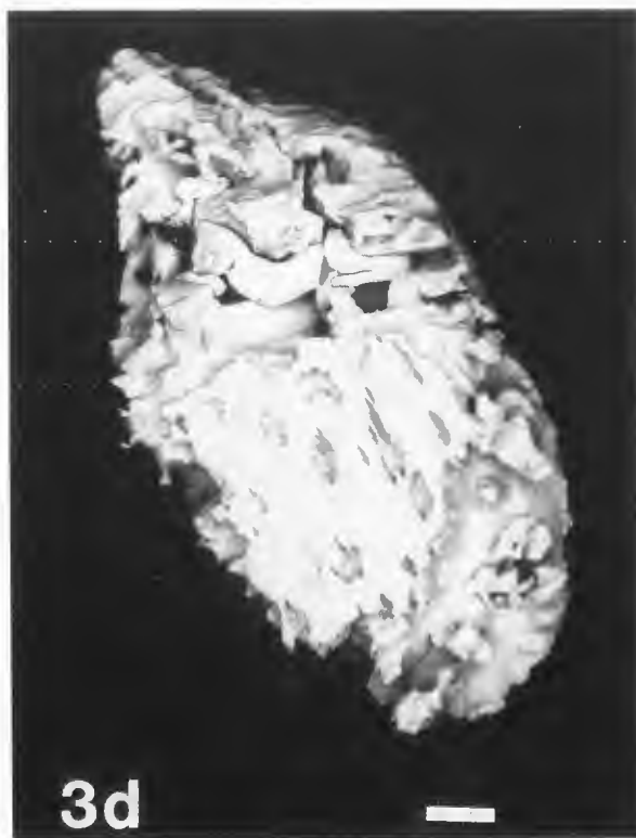
Figure 3. Backscattered electron images of four different cerussite fine-particles sampled from suspension after a residence time of 5 minutes in a solution of 0.1 N HCl. Bars = 10 \mu m.
