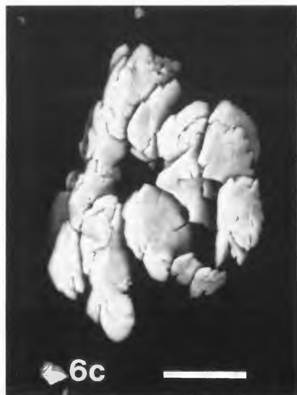
Figure 6. Backscattered electron images of two different fractured pyromorphite ( \text{Pb}_5(\text{PO}_4)_3\text{Cl} ) particles before (a and b) and following immersion (c and d) for 2 hours in 0.1 N HCl. Bars = 10 \mu\text{m} .
