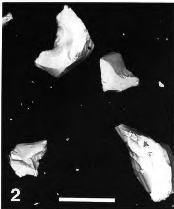
Figure 2. Backscattered electron image of fractured fine-particle cerussite ( \text{PbCO}_3 ). Bar = 100 \mu\text{m} .
