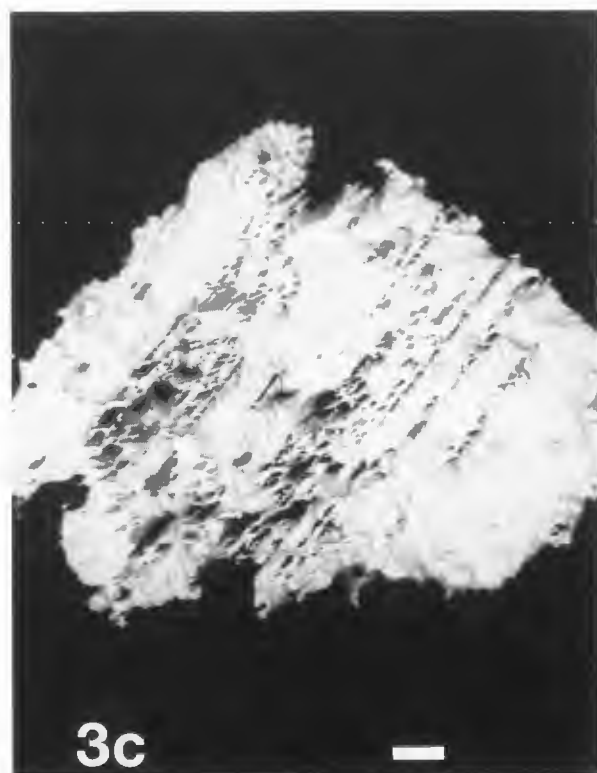
Figure 3. Backscattered electron images of four different cerussite fine-particles sampled from suspension after a residence time of 5 minutes in a solution of 0.1 N HCl. Bars = 10 \mu m.
