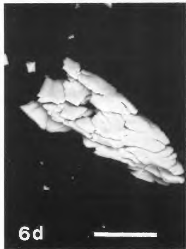
Figure 6. Backscattered electron images of two different fractured pyromorphite ( \text{Pb}_5(\text{PO}_4)_3\text{Cl} ) particles before (a and b) and following immersion (c and d) for 2 hours in 0.1 N HCl. Bars = 10 \mu\text{m} .
