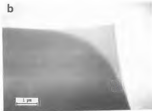
Figure 2. (a). Shape of liquid indium surface below the onset voltage for ion emission. (b). Shape of surface above the onset voltage: a Taylor-Gilbert cone has been formed.
