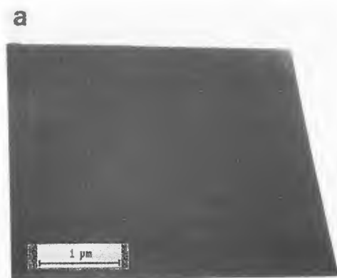
Figure 3. (a). Shape of the Taylor-Gilbert cone for an emission current of 2.8 \mu\text{A} . (b). Taylor-Gilbert cone for an emission current of 38.5 \mu\text{A} . A cusp or jet has been formed (Figures 1-3: Praprotnik, 1994).
