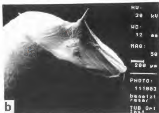
Figure 1. (a). Specimen holder for in situ TEM observations of LMIS. (b). Indium liquid metal ion emitter for in situ investigations.
