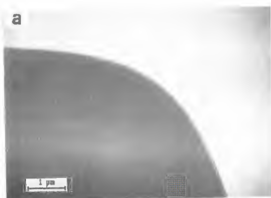
Figure 2. (a). Shape of liquid indium surface below the onset voltage for ion emission. (b). Shape of surface above the onset voltage: a Taylor-Gilbert cone has been formed.
