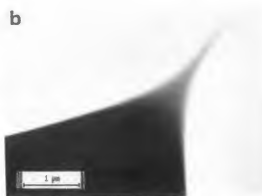
Figure 3. (a). Shape of the Taylor-Gilbert cone for an emission current of 2.8 \mu\text{A} . (b). Taylor-Gilbert cone for an emission current of 38.5 \mu\text{A} . A cusp or jet has been formed (Figures 1-3: Praprotnik, 1994).
