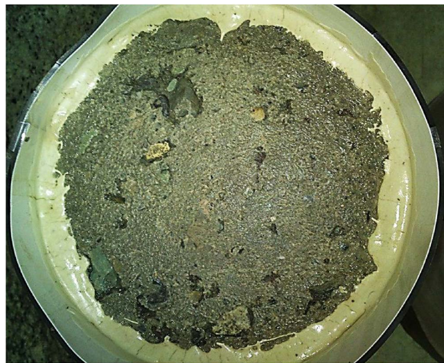
Fig. 9. T-A-32 with the air-entraining agent after 50 F-T cycles.
