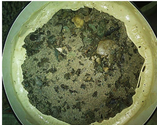
Fig. 8. T-32 without the air-entraining agent after 50 F-T cycles.
