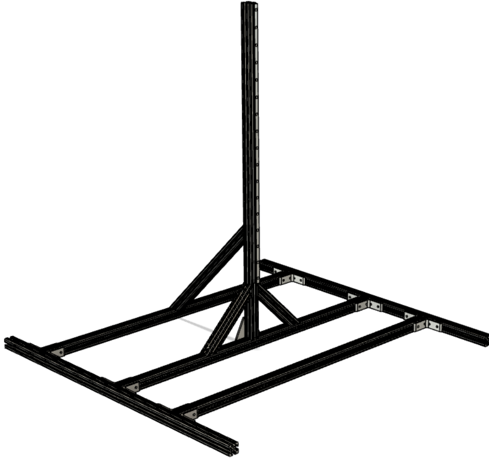
Figure 21: Final Test Stand Design, CAD Model
