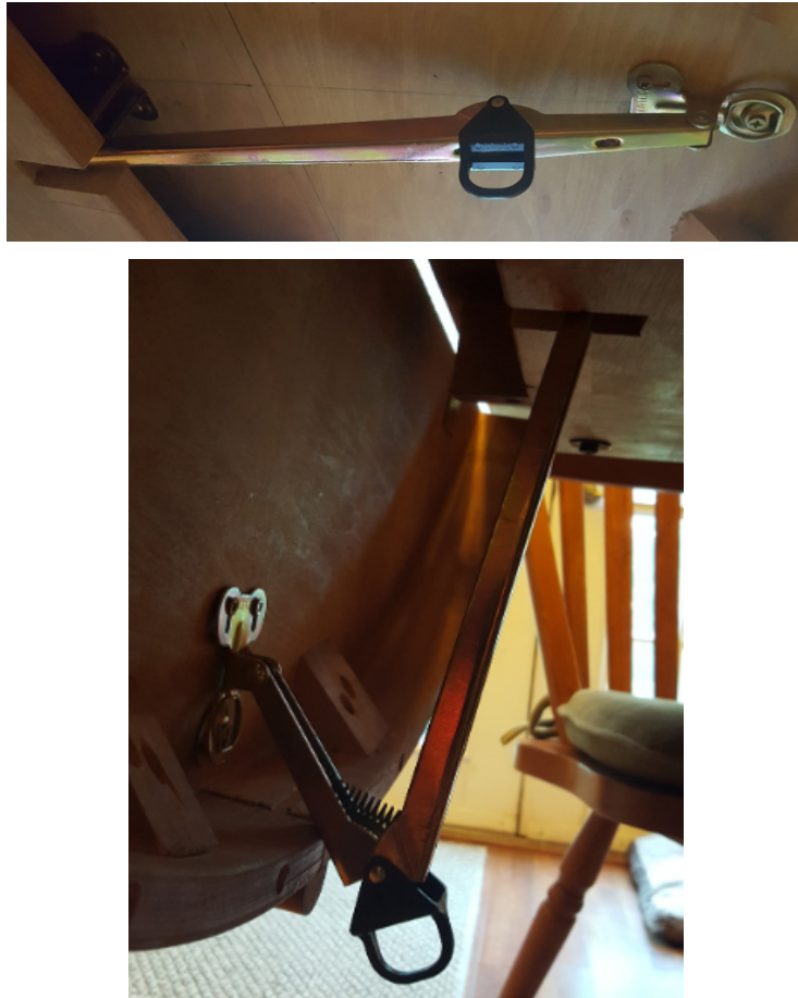
Figure D-7. Concept Prototype for Proposed Modesty Panel Support
