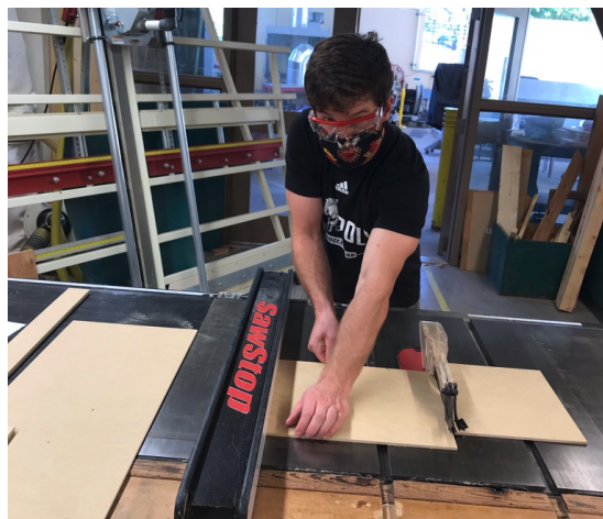
Figure 17. Cutting the Tabletops to Size on the Table Saw
