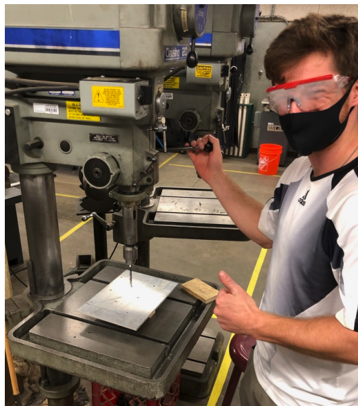
Figure 22. Adding the Hole Pattern to the Leg Spacer Plates using the Drill Press
