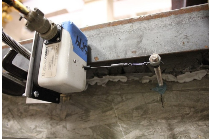
Figure 4-11: String Potentiometers, Close-up view of a typical string pot.
