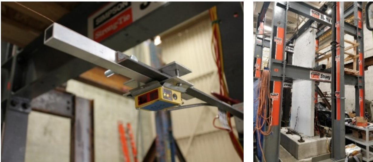
Figure 4-10: Instrumentation Column (Left) Typical optical sensor attached to a metal extension bar anchored to the instrumentation column and (Right) Instrumentation column with instruments extending out towards the wall.
