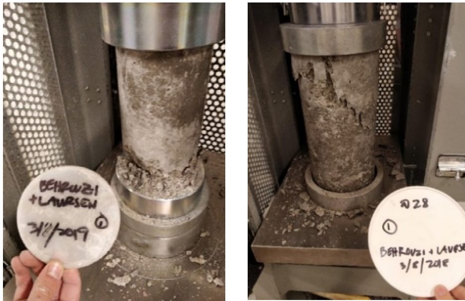
Figure 3-5: Typical Concrete Cylinder Test for Wall
