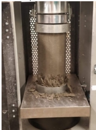
Figure 3-4: Footing Concrete Cylinder Compression Failure
