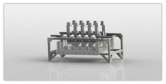
Abbott's Cardiac Rhythm Management (CRM) division tasked us with designing and building a bench test fixture to quantitatively analyze the abrasion performance of their pacemaker leads. This fixture will be used by Abbott to characterize lead abrasion against a pacemaker in the body (Lead to Can Abrasion) for their future FDA submissions.
