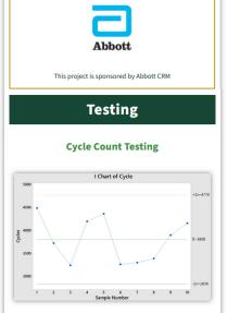
10 Abbott lead samples (sample A) were tested with our functional prototype to quantitatively characterize the lead abrasion performance. As specified in our design constraints, the relative standard deviation (RSD) for our abrasion testing must be less than 20%. The RSD is calculated by diving the standard deviation by the mean of the data.
