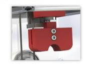
The last major mechanical requirement was to design a method of linear actuation for the lead holder. After brainstorming multiple ideas, including a rack and pinion system, we decided on a lead screw system with a load cell to ensure a precise normal force without constant stress on the stepper motor.
