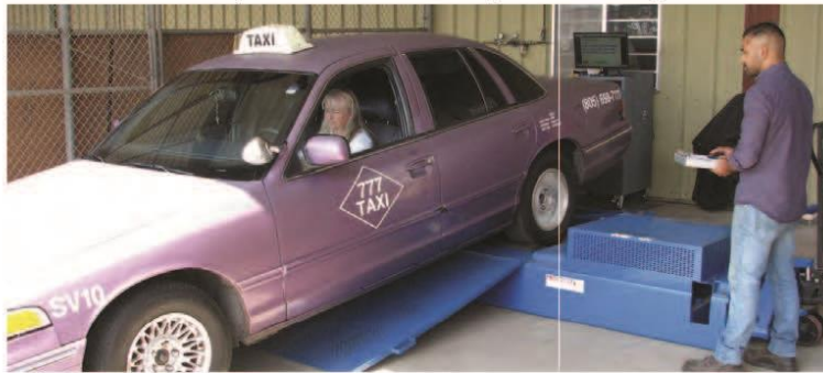
Inspector uses a Weights and Measures device to test the accuracy of a taxi meter.
