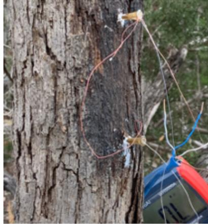
Figure 3: Sap flux sensor installation. Top needle has the heating coil, and the bottom measures the reference temperature.
