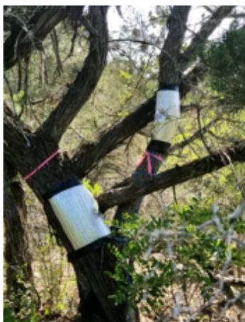
Figure 4: Sap flux sensors installed and covered by reflective thermal insulation.
