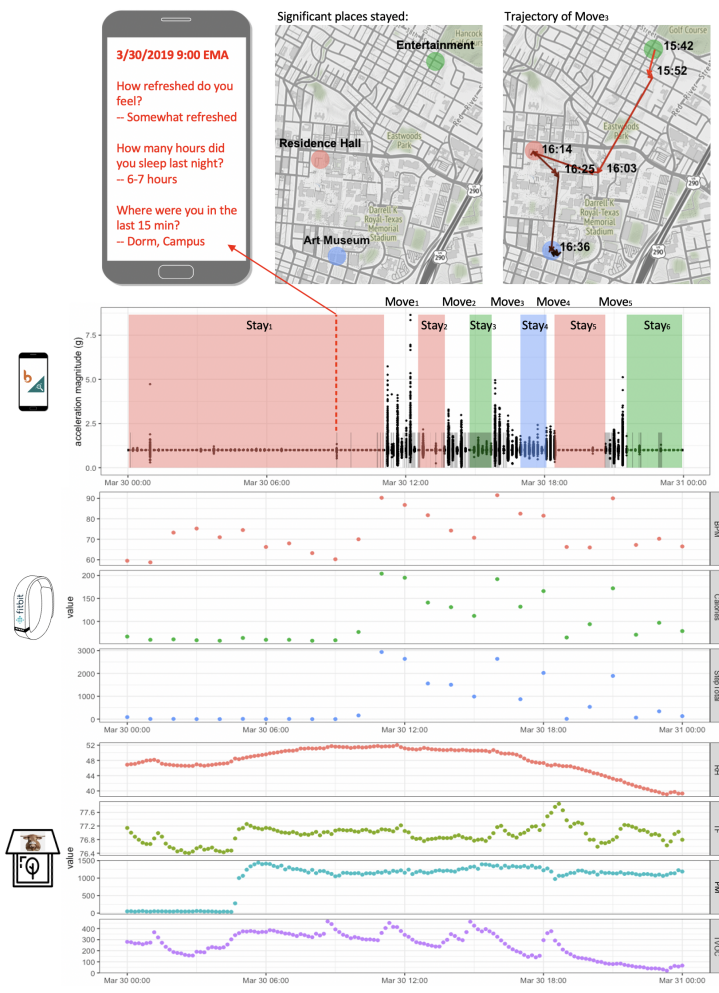
Figure 3: Data collected from the smartphone, Fitbit, and BEVO Beacon of an example participant during a given day (March 30th 2019). Plotted data modalities are: EMA (questions and answers shown against phone image background on top), GPS (clustered significant places and an example movement trajectory shown in maps on top and as vertical bands), accelerometry (black dots), screen activity (short grey bands), heart rate (BPM), calories spent in the past hour (Calories), steps taken in the past hour (StepTotal), home relative humidity (RH), home temperature in degrees Fahrenheit (TF), home particulate matter in \mu\text{g}/\text{m}^3 (PM), and home TVOC (TVOC).
