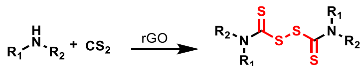
Scheme 1.10: rGO catalyzed the bis(aminothiocarbonyl)disulfides in one-pot.
