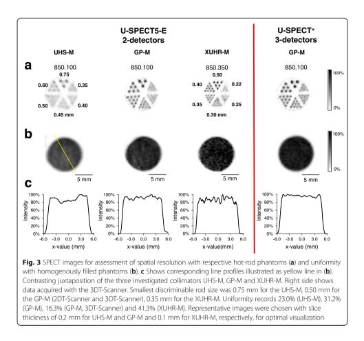
The 3DT-Scanner achieved a uniformity of 16.3% with the GP-M collimator and was therefore superior to all collimators examined in 2DT-Scanner. Reconstructed images and line profiles are shown in Fig. 3a, b for illustration.
