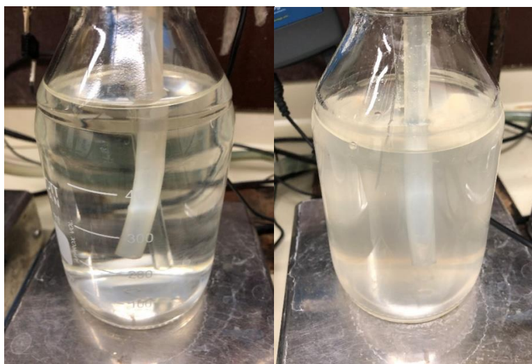
Figure 8. Appearance of synthetic media on set 2 at start of experiment (left) and cloudiness after 15h of experiment (right).
